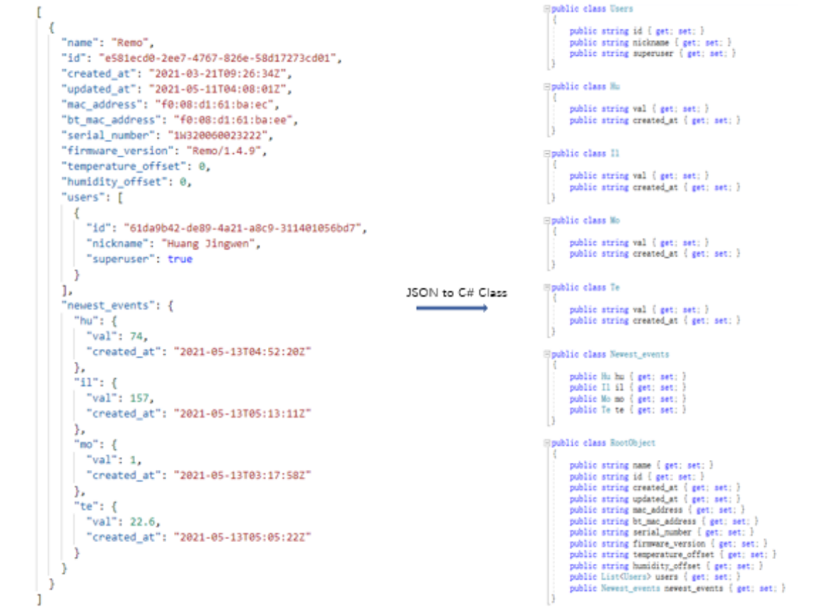
Fig. 6.8 Conversion of JSON data into C# classes
